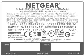
Figure 5. Switch label model XS724EM
